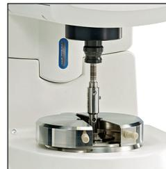
*Thermal Barrier reduces the effects of heat transfer to the environment. Two part chamber provides thermal isolation of the measurement zone.*
